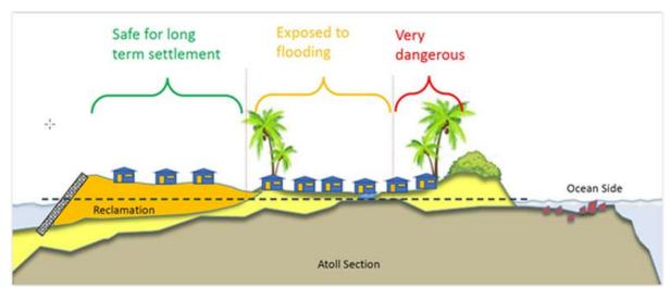
Source: Arthur Webb (TCAP). This schematic diagram shows the model of coastal adaptation, with particular emphasis on coastal reclamation, being used in Tuvalu as a way to counter future Sea Level Rise.
